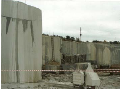
Fig 3: Diamond wire-cutter in operation
